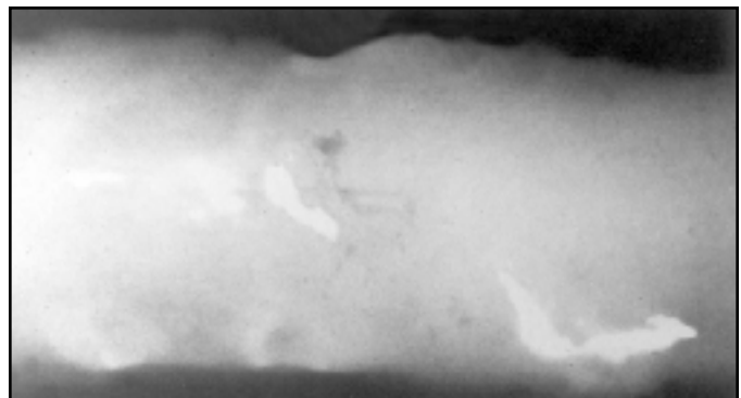
Figure 15: Radiograph Showing Copper Contamination (Copper contamination shows up as lighter and irregularly shaped areas.)
