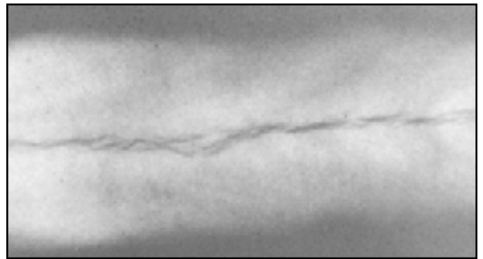
Figure 11: Radiograph Showing Longitudinal Weld Cracking
