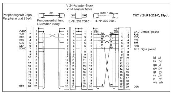
With this wiring type only transfer stop with DC3 (software handshake) is possible!
