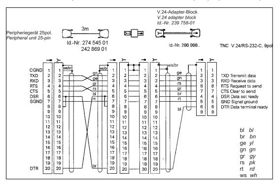
If the pin layout of your peripheral unit differs from the above, the HEIDENHAIN connecting cable cannot be used.
