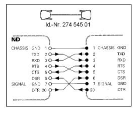
Diagram no.17 V.24/RS-232-C direct connection for softw. handshake, ND/PT 25-pin / peripheral unit 25-pin
