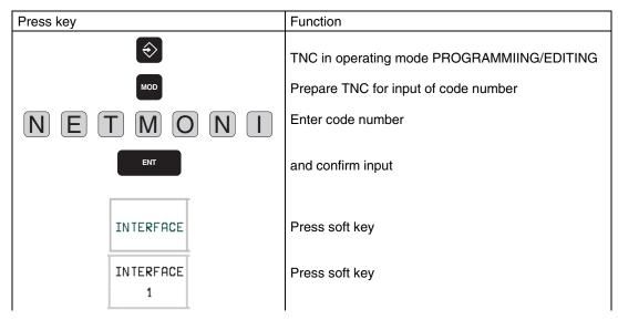
The hardware address of the Ethernet card is now displayed on the screen: INTERFACE IS ETHERNET XX:XX:XX:XX:XX.
