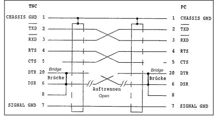
This modification applies for hardware handshake with TNC 145 to TNC 155. In these control models, the RTS pin is not connected but tied high internally. The following modification is required for hardware handshaking:
