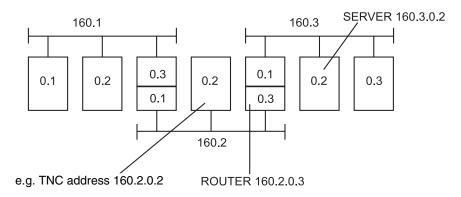
The boxes represent for example TNCs or personal computers. Please observe that a TNC can never be a ROUTER, since it does not feature the second connector for feeding signals through.
