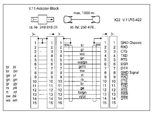
The pin layout of the RS-422-/V.11 data interface **is the same** at the logic unit X22 and at the V.11 adapter block.
