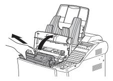
While holding the green lever, flip the transfer guide up. Gently ease the edge of the paper away from the guide. After the paper rear-most edge has come out, slowly pull the paper forward and out of the fax unit.
