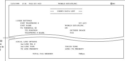
After you have installed the optional Dual-line Upgrade Kit II, the settings selections you register for Line 2 will appear in the User Data List. (-16-32)
