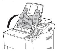
3. Open the printer cover and remove the toner cartridge. Store the cartridge in its original protective bag to avoid exposure to light.
