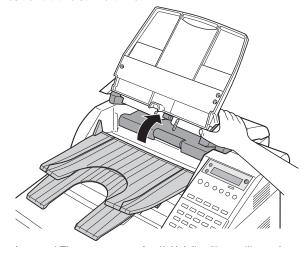
7. While holding the ADF cover open with one hand, use one finger of your other hand to gently push in the black plastic loop to separate it from the stub on the fax machine.
