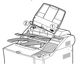
☐ Attach the supplied tray labels as shown in the illustration below. We also recommend attaching the tray labels onto the upper and lower output trays according to the settings you make on the SELECT OUTPT TRAY menu to classify the outputs. (→2-52) You can use the blank labels to meet your specific needs.
