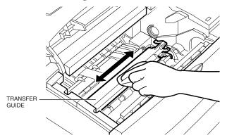
5. While holding the green lever, flip the transfer guide up. Wipe the edge of the transfer guide with a soft, clean cloth, to remove toner and paper dust from both sides of the transfer guide.
