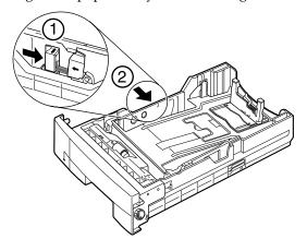
Push up the stopper of the paper size rear guide, and slide it to the mark indicating the desired paper size.
