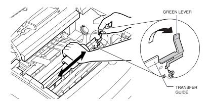
6. Pull the transfer guide back to its full extent, then wipe the silver metal strip with cloth. Then gently guide the transfer guide back to its original position.
