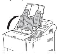
2. Open the printer cover and remove the toner cartridge. Store the cartridge in its original protective bag to avoid exposure to light.
