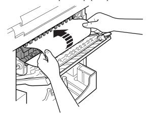
3. After the paper's edge has rolled out, pull the paper forward carefully.
