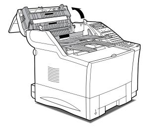
9. Use a soft, dry cloth to wipe clean the scanning glass, the white strip above, rollers and the area around the glass. Use a soft cloth that will not scratch the scanning glass.
