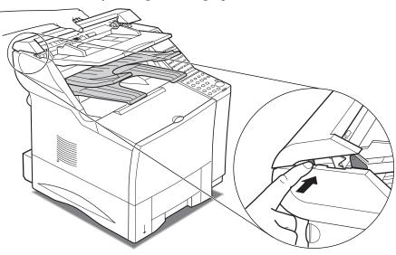
Open the upper unit of the ADF cover fully and clean the rollers.
