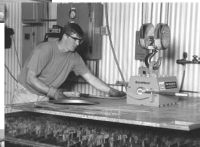
The Eriez Heavy-Duty Rectangular Magnet is effective in single or multiple-magnet applications for handling heavy fabrications or for lifting several thicknesses of sheet or plate at one time.
