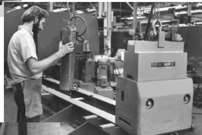
Heavy-Duty Rectangular Magnets provide maximum efficiency in multiple-plate handling applications like this.
