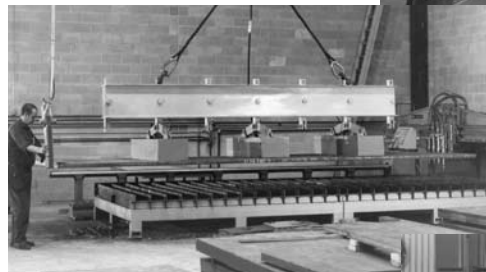
A Safehold® Permanent Magnet makes many lifts practical even with only minimum contact.
