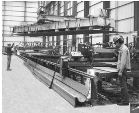
Eriez Bi-Polar Magnets, with a wide range of optional pole-plate configurations, are ideally suited for handling pipe, rounds, bundles, angles and shapes. They can be used in single- or multiple-magnet applications.
