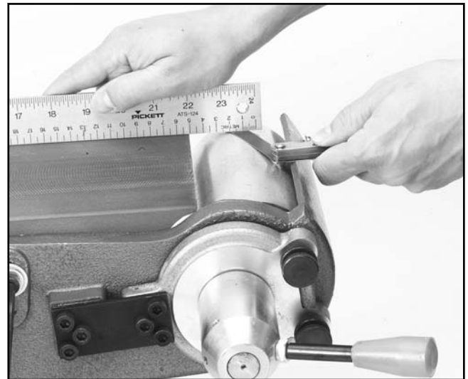
Figure 15. Measuring platen to roller parallelism.
