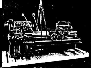
Wood block A is taken from the skid and blocks B should be wide enough to keep the sling clear of the leadscrew reverse rod.
