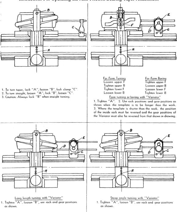
Instructions For Operating the Anti-Friction Bearing Taper Attachment
