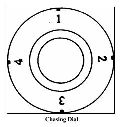
For half threads engage the halfnut at opposite graduations, as for instance No. 1, or No. 3, or No. 2, or No. 4. For quarter threads engage the halfnut at the same graduation each time. For other fractional threads the use of the thread chasing dial is not recommended.
