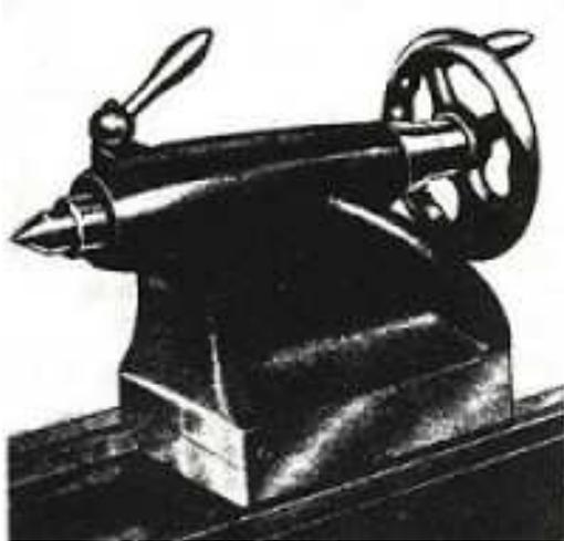
The Tailstock is of rigid design with a large diameter spindle and screw, and is mounted on independent vee and flat surfaces on the bed. The hole in which the spindle slides is honed to very close limits of accuracy.
