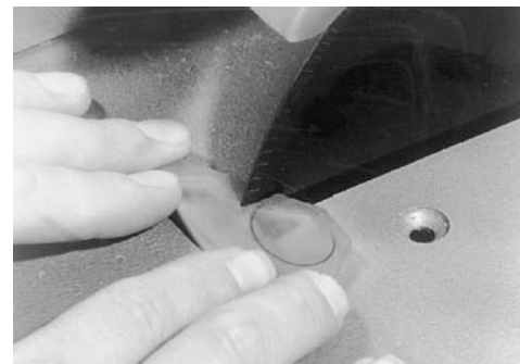
4. All cuts must be made in a straight line. Be careful not to put side pressure on the blade. Successive straight cuts approximate curved lines that will be finished on a grinding wheel. Make all trim saw cuts outside the template mark.
