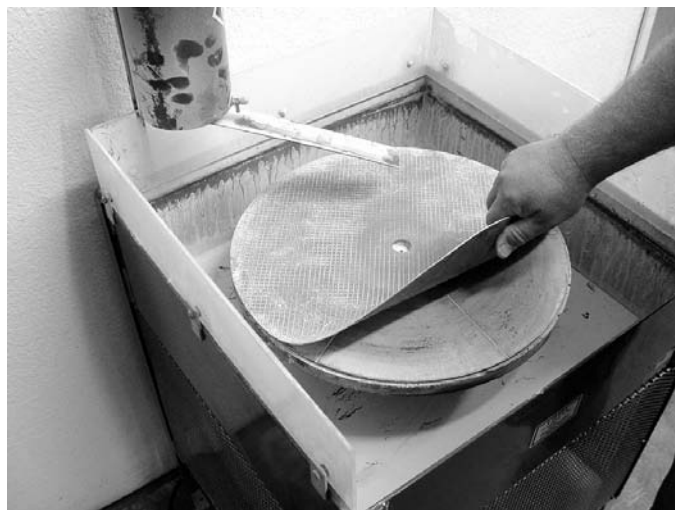
Shown above is Magnetic Nova being removed from an 18RLD lap machine.
