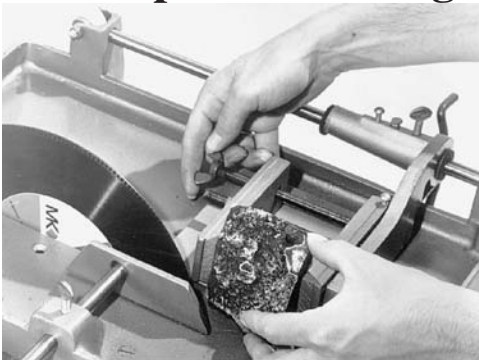
1. Object to be slabbed is clamped in vise. The cut is started by hand pressure.
